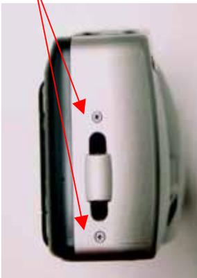
Remove screw from door latch side
