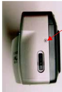
Remove screw inside camera enclosure
