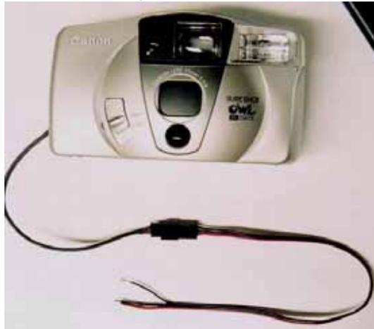
"Film" winding will be heard after the first test. Subsequent test will not include winding without film in the camera. A 6 second delay is needed between tests for the flash capacitor to recharge.
