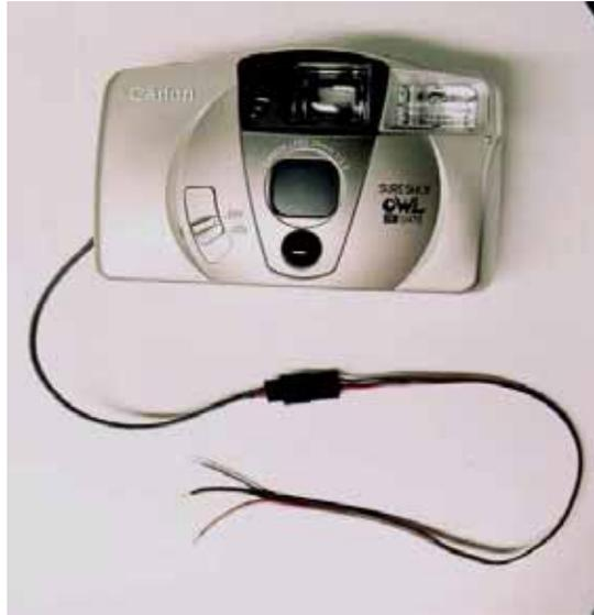
To test camera, refresh wire #6 and shutter wire #5 are solder together. Camera will fire flash when these two wires are touched to common wire #4. Camera must be on, and back door must be latched.
