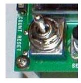
There are 3 selectable setting to control the trigger pulse of the HH1 Kit to the camera.
